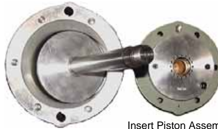
Insert Piston Assembly into the bore at a 45 deg. Angle and straighten it so that the Piston assembly is at the bottom of the bore
